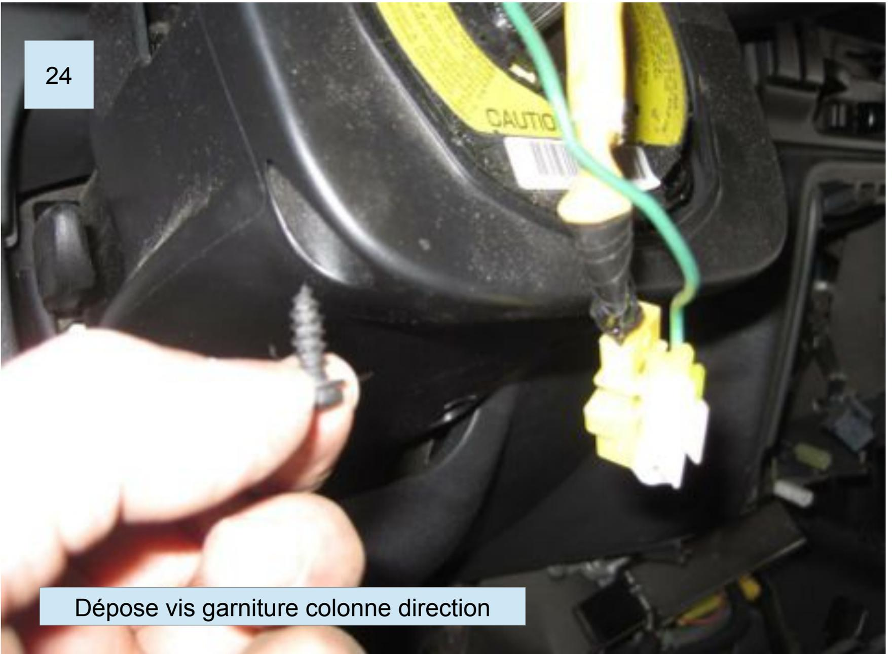
Dépose vis garniture colonne direction
